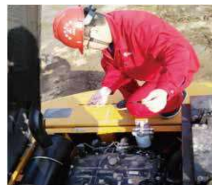
Inspect the situation of engine oil
