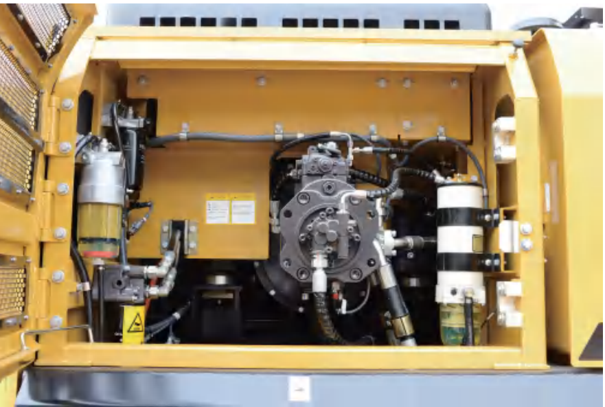
Large-capacity multi-stage filter system
